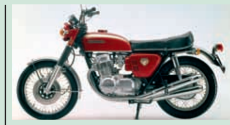
1969 First mass-produced motorcycle with disk brakes (Honda CB 750 Four)
