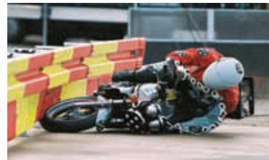
Safety integrated into the landscape: NATURE rail with underrun protection was designed especially for equipping winding biking roads. Flexible underrun protection prevents motorcyclists from sliding under the safety barrier.
