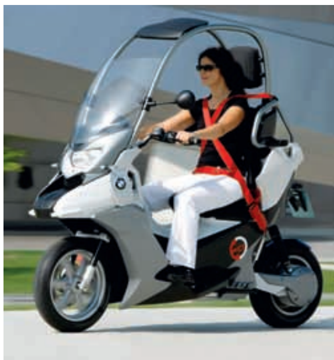
With the BMW C1, the rider is protected by an enveloping yoke structure.
